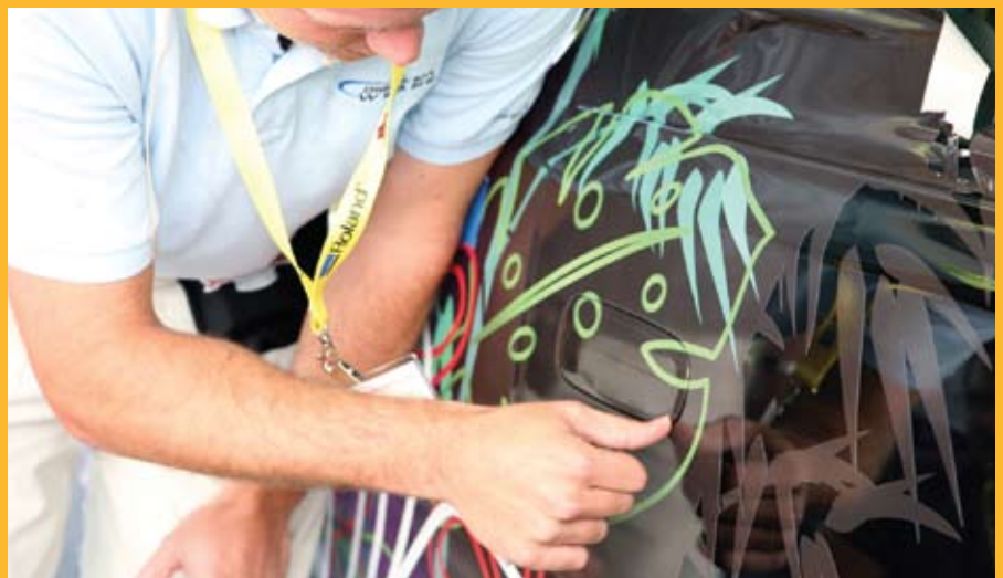
Door handles and other complex surfaces can present challenges during the installation process.
